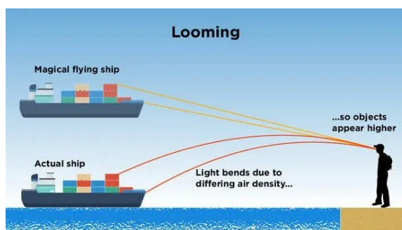
Figure 11: Total Internal Reflection in Looming
